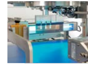
Blade cleaning unit with uv-c-light
