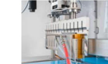
Blade cleaning and washing unit
