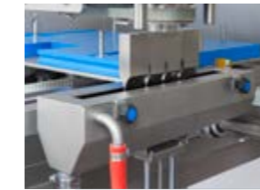
Blade cleaning and washing unit
